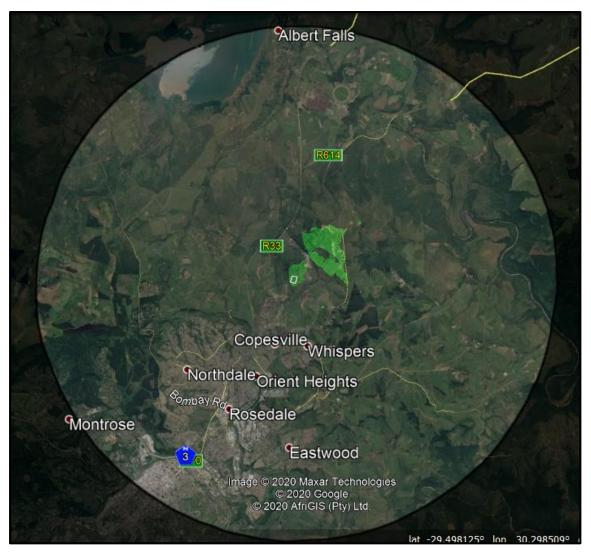
Figure 34: Viewshed of S1 where the green shaded areas indicate the positions from where the lowest point of the earmarked area (white polygon) will be visible. (Image obtained from Google Earth).
