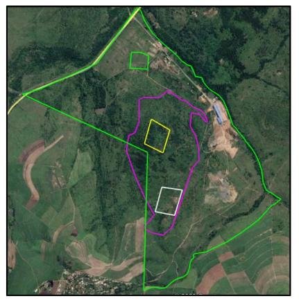
Figure 37: Rough estimation of the proposed dolerite intrusion (pink polygon) on the earmarked property, where the white polygon indicates S1, and the yellow polygon S2. (Image obtained from Google Earth).
