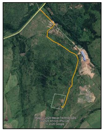
Figure 3: Satellite view showing the path of the existing access road (orange line) to the proposed mining area (white polygon).
