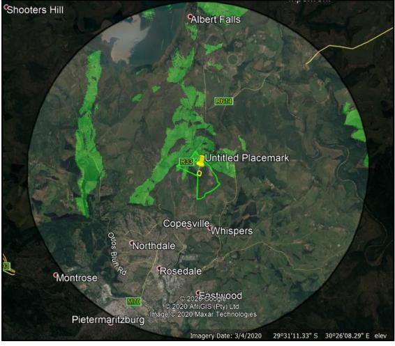
Figure 36: Viewshed of S2 where the green shaded areas indicate the positions from where the lowest point of the earmarked area (yellow polygon) will be visible. (Image obtained from Google Earth).
